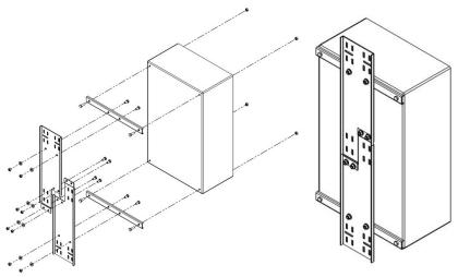
**STEP 4:** If pole mounting the enclosure, assemble the pole mount kit to the back of the enclosure and mount the enclosure to a pole using the 6 hose clamps provided. The enclosure can also be wall mounted using the 4 holes in the back of the enclosure.
