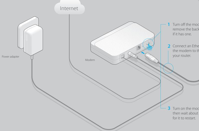
1 Turn off the modem and remove the backup battery Router
