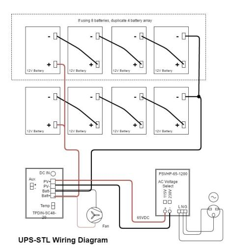
**STEP 7:** Before attaching the battery cables to the batteries, first remove the battery cable fuse. This will prevent accidental short circuit.
