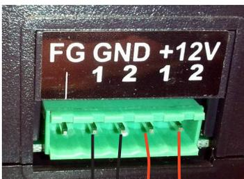
**FG** = Frame Ground (Do Not Connect to V-)
