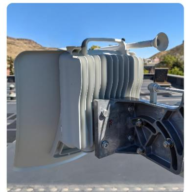
**Note:** It is recommended to use a precision mount bracket to setup the link. A bracket provides more granular control for fine-tuning azimuth and elevation angles.
