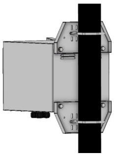
**Note:** There are multiple cable gland feedthrough in the bottom of the enclosure. If you are not using any of the feedthrough you can cut a short piece of wire, put it through the cable gland and tighten the cable gland on the wire to seal it.
