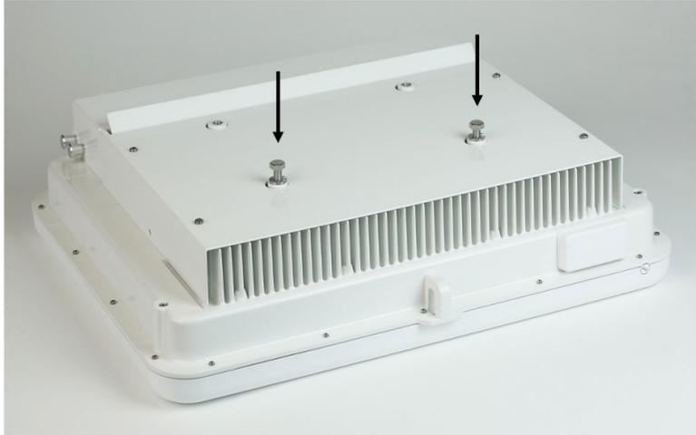
The BN must be slid into the top slots on the bracket ears using these two bolts.
