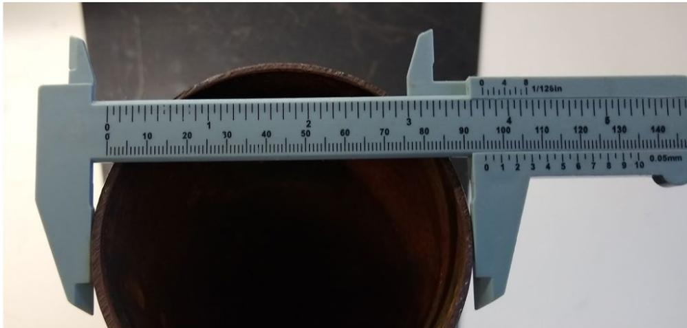
Figure 4: Measure Pole Diameter
