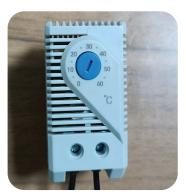
Adjust the temperature controller pointer back to 0 scale when making power-on test
