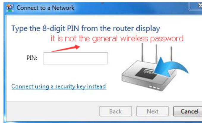
2. If you cannot find the PIN or PIN failed, you may choose [Connecting using a security key instead](#), and then type in the [Wireless Password/Network Security Key](#);
