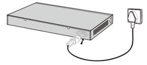
Figure 4-3 Connecting to Power Supply
