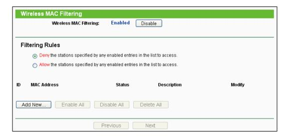
Figure 6-11 Wireless MAC Filtering
