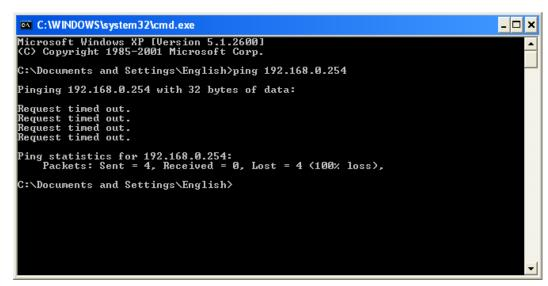
Figure 3-2 Failure result of Ping command
