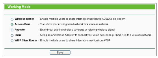
Figure 5-7 Wireless Working Mode Settings
