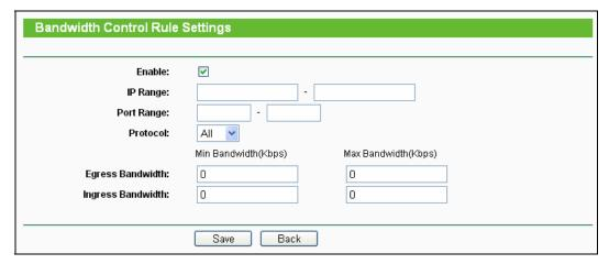
Figure 4-79 Bandwidth Control Rule Settings
