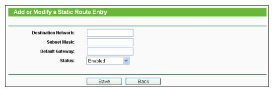
Figure 4-74 Add or Modify a Static Route Entry
