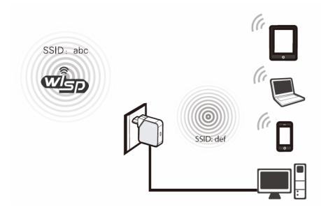
Figure 2-5 Hardware Installation of the TL-WR710N in WISP Client Router Mode
