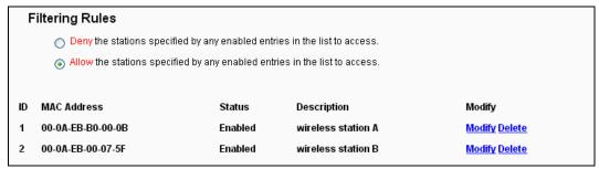
Figure 4-25 Filtering Rules
