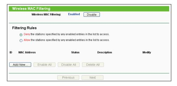
Figure 8-19 Wireless MAC Filtering
