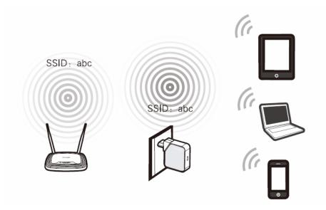
Figure 2-3 Hardware Installation of the TL-WR710N in Repeater Mode
