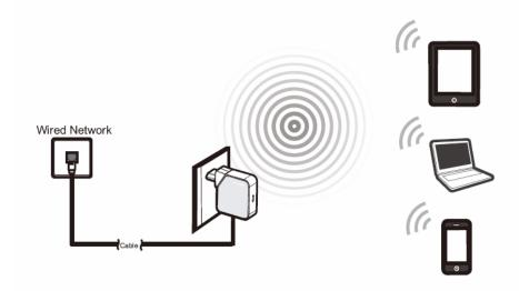
Figure 2-2 Hardware Installation of the TL-WR710N in AP Mode
