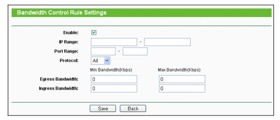
Figure 8-75 Bandwidth Control Rule Settings
