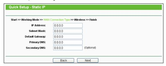
Figure 3-22 Quick Setup - Static IP
