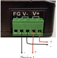
FG = Frame Ground. Connect to Earth Ground
