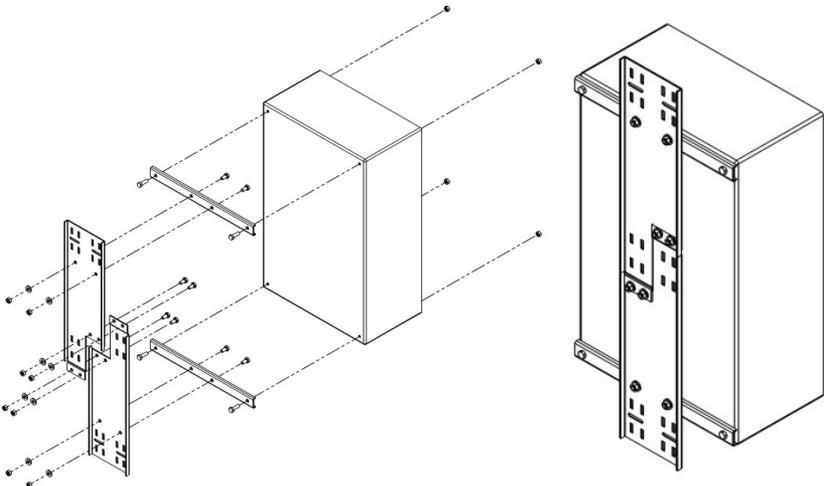
**STEP 4:** If pole mounting the enclosure, assemble the pole mount kit to the back of the enclosure and mount the enclosure to a pole using the 6 hose clamps provided. The enclosure can also be wall mounted using the 4 holes in the back of the enclosure.
