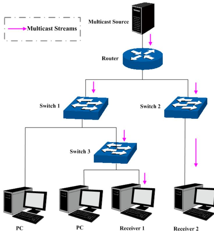
Figure 8-1 Information transmission in the multicast mode
