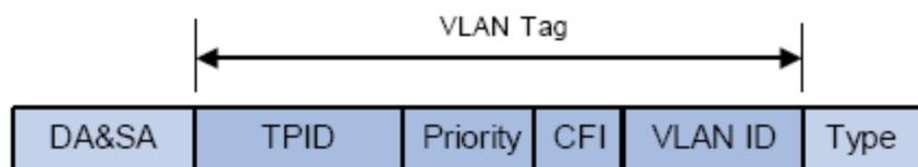
Figure 6-2 Format of VLAN Tag
