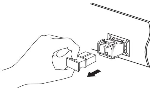
4. Plug a fiber-optic cable into the SFP. Note that the SFP works without any additional configuration.
