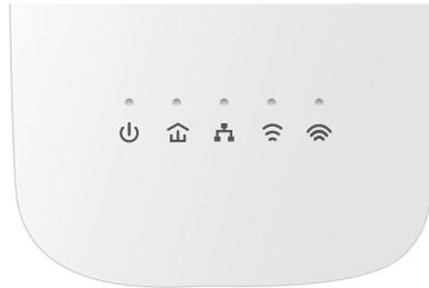
LEDs of the extender are located on the front side. They indicate the working status. For more details, please refer to the following table.
