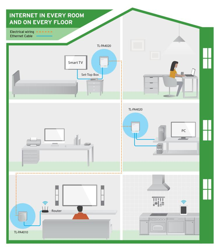
To achieve maximum performance, 500Mbps powerline adapters should be paired with adapters featuring no less than 500Mbps powerline data transmission rates.
