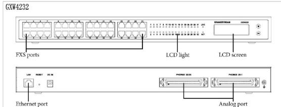
Here is the example for GXW4232. GXW4216 and GXW4224 are connected in the same way.
