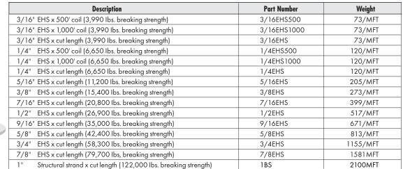
To arrive at safe working load for guy wire appropriate safety factor must be applied.
