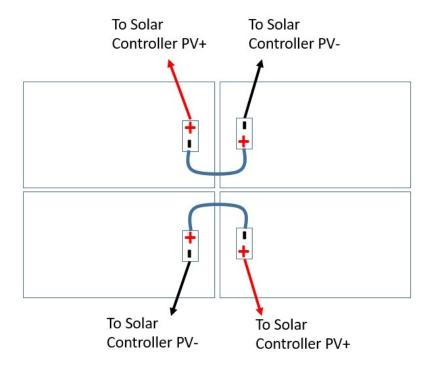
**STEP 9:** Once the batteries and solar panels are all connected and wired to the Large Green Connector, Disconnect PV+ wire and plug the connector to the MPPT Solar Controller until the connector latches click into place. The Battery Charging LED should light up for about 60 seconds. Now connect PV+ to the green connector.
