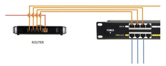
Connect the LAN port to your Ethernet switch. This device handles all 10/100/1000 mb modes - so all gigabit and fast Ethernet switches are compatible. Power is provided on the POE ports on pins 1 and 2 (minus) and 3 and 6 (plus) and also on pins 4 and 5 (plus) and 7 and 8 (minus).
