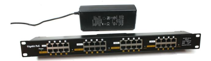
This device injects power onto gigabit data connections. 48 Volts is available all the time, there is no autonegotiation with the attached client device. This device has no switching function – there is no configuration needed, and VLANs and other management features of any switch will be handled transparently thru the injector.
