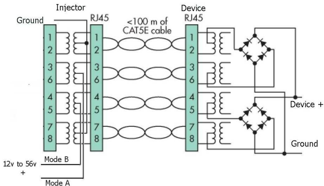
As you can see – the Client devices have diode bridges – this allows for cross over cables to be used in the wiring infrastructure. Also notice – that because of 488A and 488B pinouts – it makes no difference if pins 12 and 36 polarity is exchanged.
