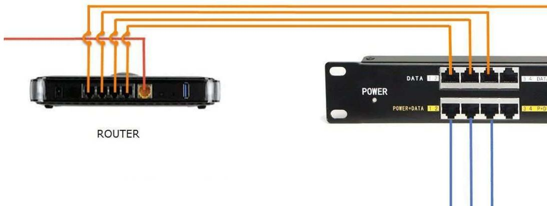
Connect the LAN port to your Ethernet switch. This device handles all 10/100/1000 mb modes – so all gigabit and fast Ethernet switches are compatible. Power is provided on the POE ports on pins 1 and 2 (minus) and 3 and 6 (plus) and also on pins 4 and 5 (plus) and 7 and 8 (minus).
