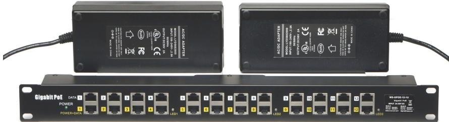
This device injects power passively. 56 Volts is available all the time, there is no autonegotiation with the attached client device. This device has no switching function – there is no configuration needed, and VLANs and other management features of any switch will be handled transparently thru the injector.
