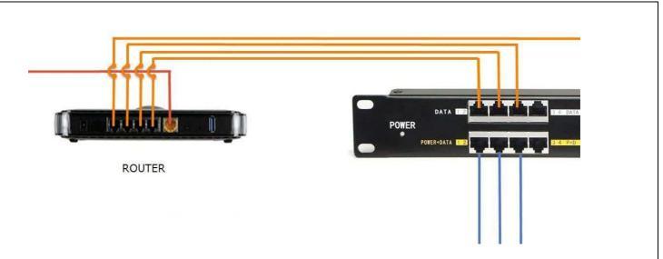
Connect the LAN port to your Ethernet switch. This device handles all 10/100/1000 mb modes – so all gigabit and fast Ethernet switches are compatible. Power is provided on the POE ports on pins 1 and 2 (minus) and 3 and 6 (plus) and also on pins 4 and 5 (plus) and 7 and 8 (minus).
