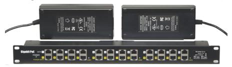
This device injects power passively. 56 Volts is available all the time, there is no autonegotiation with the attached client device. This device has no switching function – there is no configuration needed, and VLANs and other management features of any switch will be handled transparently thru the injector.
