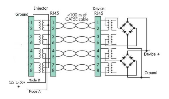
As you can see – the Client devices have diode bridges – this allows for cross over cables to be used in the wiring infrastructure. Also notice – that because of 568A and 568B pinouts – it makes no difference if pins 12 and 36 polarity is exchanged.
