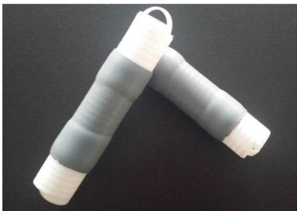
CST-M series weatherproofing solution is a cold shrink tube with built-in mastic. It is a one-step, time-saving and reliable weatherproofing design. The innovatively unique design economically protects RF coax connections at wireless cell sites and CCTV networks against water, dust, and other environment corrosion in a quick, reliable and safe way.
