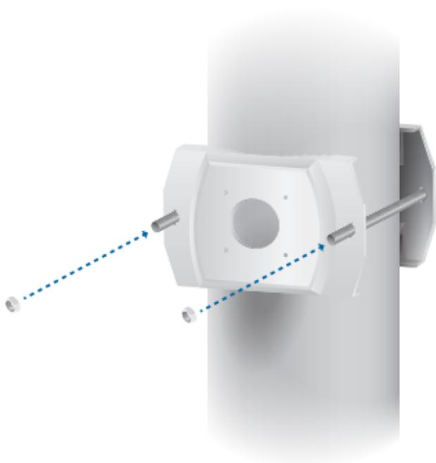
3. Position the camera in front of the appropriate *Mounting Bracket*. Then feed the cable through the opening.
