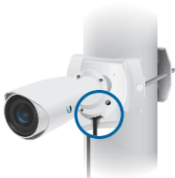
*Cable Feeds through the Bottom Slot of the Camera*
