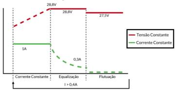
The graph above shows the charging stages of the battery charger, illustrating the behavior of the voltage and current of the batteries as well as the migration point from one stage to the next. Current values might vary depending on the source model
