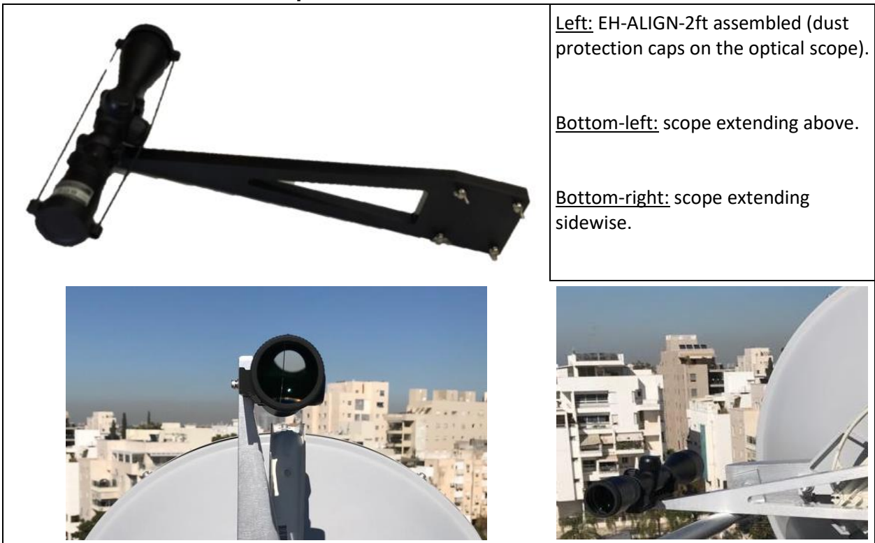
FIGURE 2: Assembled scope mounted on 2ft antenna
