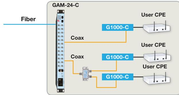
Since the G.hn Access Network operates at layer-2 (same as Gigabit Ethernet and GPON), the G1000-M and G1000-C can operate under a virtual CPE (vCPE) mode when Operators rely on a Virtualized Network Function (VNF) architecture where services such as IP Routing and Firewall are handled by servers in the “cloud”.
