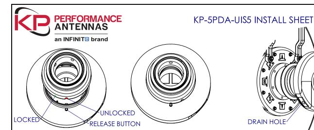
1. Attach Ubiquiti radio to adapter and align larger, UNLOCKED indent with radio's RELEASE BUTTON. Slot in adapter and rotate to smaller, LOCKED indent. To remove radio, press RELEASE BUTTON and rotate adapter to UNLOCKED indent.
