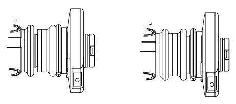
4. Pull back collar on Quick-Connect Waveguide Coupler and slide adapter over feed assembly. Release coupler.
