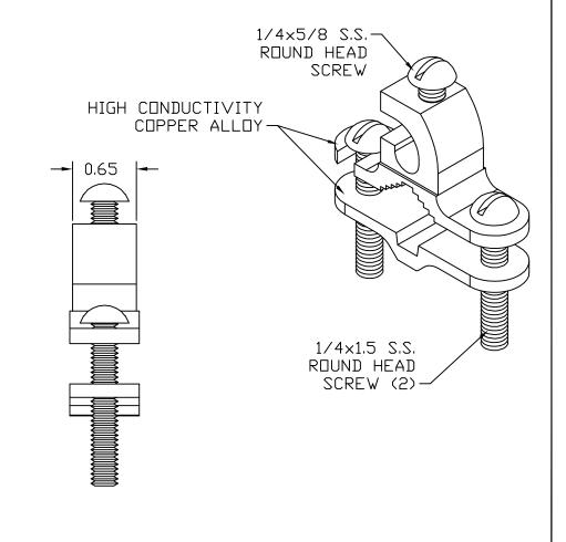
SUITABLE FOR DIRECT BURIAL IN EARTH AND CONCRETE
