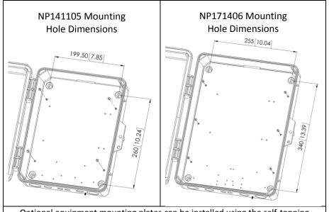
Optional equipment mounting plates can be installed using the self-tapping screws provided with your Altelix enclosure. Metallic and non-metallic plates can be purchased at <a href="https://www.altelix.com">www.altelix.com</a>.
