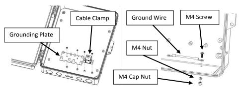
Cable clamp and grounding plate can be installed using the provided self-tapping screws
