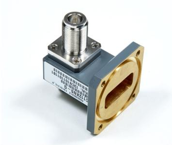
Waveguide/Coaxial Cable Transition for WR137, 5.85–8.2 GHz, with interface types N Female and CPR137G, gray
