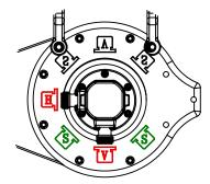
Align adapter with feed assembly's input waveguide. Rotate adapter such that direction of connectors is aligned with H/V (Horizontal/Vertical) or \$/\$ (+/- 45 Slant) indicators on the back of the antenna.
