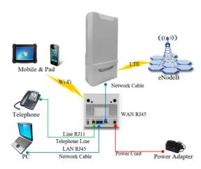
GWG-136WV provides 1 PoE WAN, 2 Gigabit LAN Ports, 1 RJ11 phone port, high performance 802.11b/g/n/ac dual band Wi-Fi and software firewall for security, providing an effective all-in-one solution to SOHO or residential customers.
