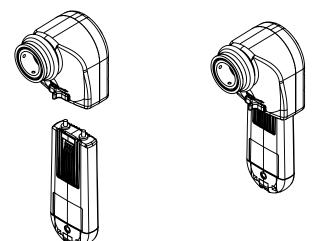
1. Push Cambium radio into the adapter until it locks into place. To release the radio, slide tab to the open position.
