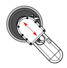
3. For horizontal/vertical polarization, align the radio to point up-down. For +/- 45 Slant polarization, align the radio at a 45 degree angle.
