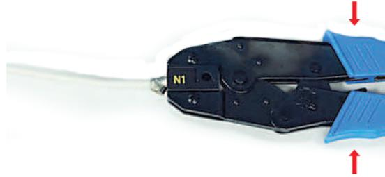
2. Squeeze the tool to push the contact blades into correct positions.
