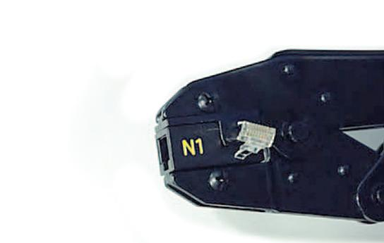
5. Squeeze the tool again for holding the cable tightly and grounding.
