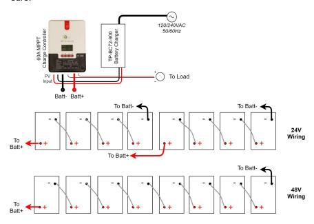
**STEP 2:** Place enclosure on the foundation. Install 8 batteries in the box. Use a rope tied to the battery tabs to lower batteries into the box. Connect all 8 batteries in series configuration for either 24VDC or 48VDC (See Wiring Diagram Below and near the end of this booklet)
