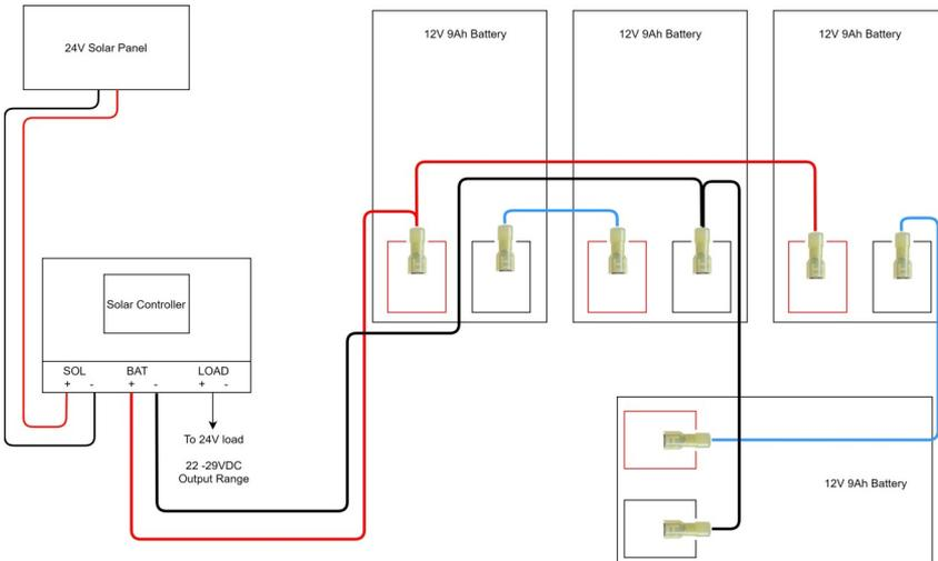
systems don't require any maintenance. They should last up to 5 years in normal use. **Note: Never store batteries for any length of time in a discharged state or it will damage the battery.**
