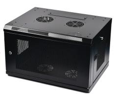
The side panels and front door lock securely to help prevent damage, tampering or theft. The front, top, bottom and removable side panels are vented, which allows air to flow freely and keep equipment cool. The reversible front door can open left or right by rotating the cabinet 180° before mounting. Convenient top and bottom ports allow easy cable routing.
