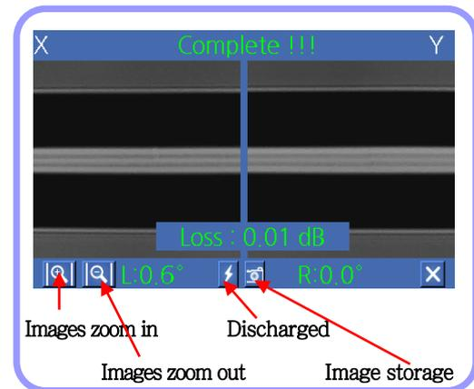
If the measured cut angle or computed loss value is greater than the preset limit, an error message appears on the screen. Also, an alarm can be triggered by the discovery of an abnormal condition of the spliced part including too thick or thin area or bubbles. Even if an error message does not occur, it is recommended to perform the arc fusion process again if the result on the screen does not look good enough when examining it with naked eyes.
