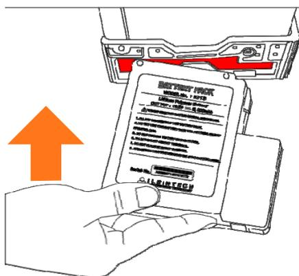
Insert the battery pack into the battery groove until it clicks.
