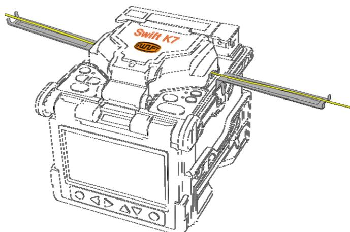
Install the cooling tray on the rear side of heater as follows.
