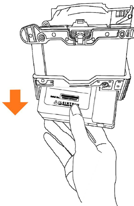
Please make sure the power is off before removing the battery. Remove the battery by releasing lock lever.
