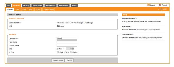
Note when setting the connection mode as L2 Bridge or L3 Bridge, there will be a warning window pops up. Remember the management IP address 192.168.0.1 and click the "ok" button.
