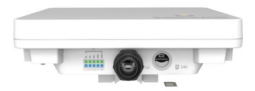
Open the SIM card cover, insert the SIM card and connected the ETH cable.
