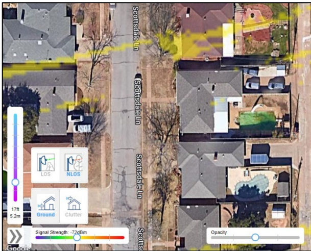
Height & signal strength sliders allow dynamic control of coverage for the heat map.
