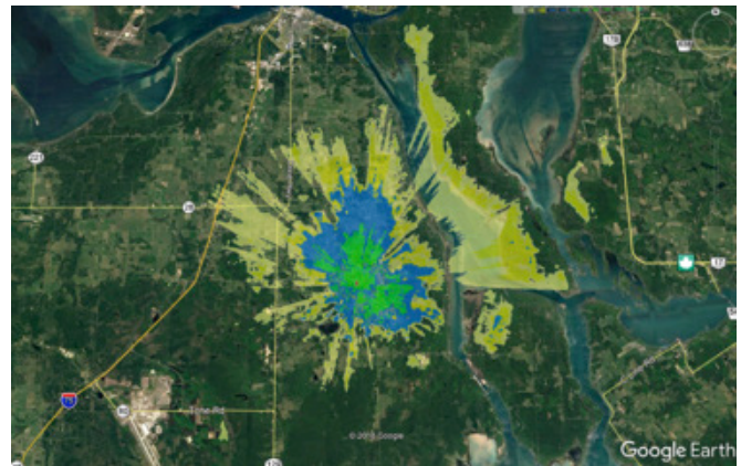
Figure 2: TVWS 18dBm Tx, 30M tower & 8M remote
